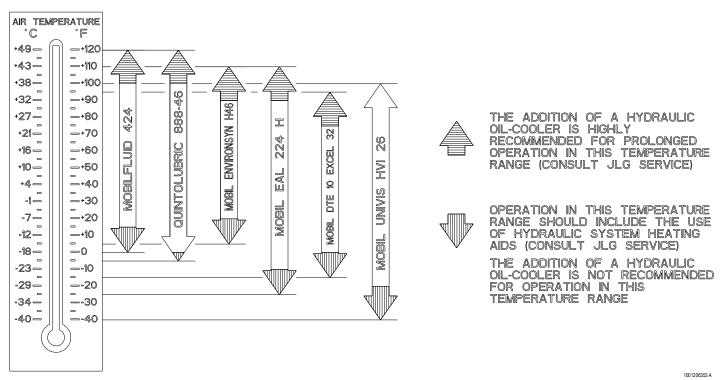
Figure 7-4. Hydraulic Oil Operation Chart - Sheet 1 of 2
