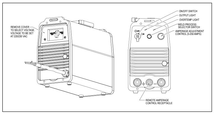
Figure 6-2. SkyWelder™ - Sheet 2 of 2
