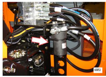
Lube Point - Replaceable Element Interval - Change after first 50 hours and then every year or 600 hours of operation, whichever comes first
