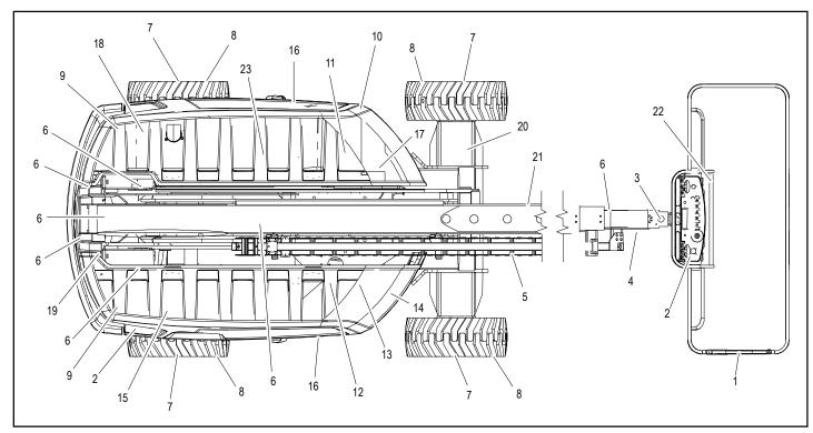
Figure 2-3. Daily Walk-Around Inspection Diagram
