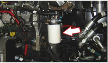
Lube Point(s) - Replaceable Element Interval - 600 hours of operation
