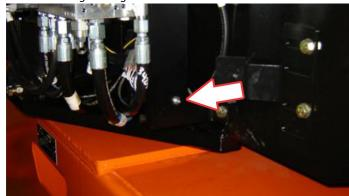
Lube Point(s) - 1 Grease Fittings Capacity - A/R
