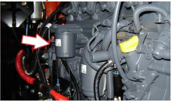
Lube Point(s) - Fill Cap/Spin-on Element
