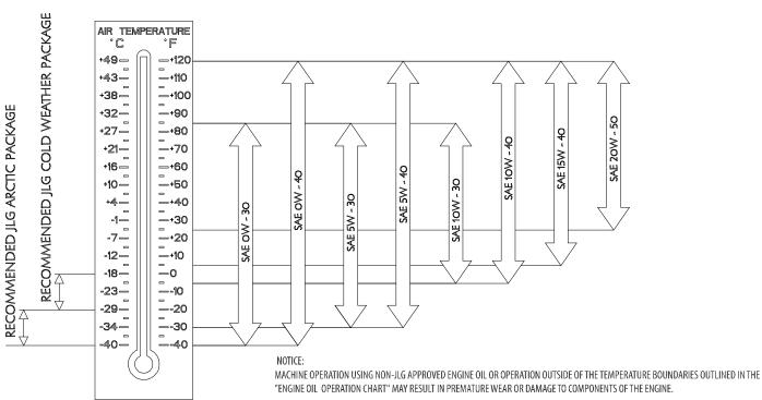
Figure 7-3. Engine Operating Temperature Specifications - Deutz 2011
