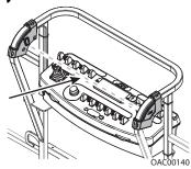
Reattach magnetic end of cable to bracket if it becomes disconnected.
