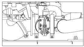
Figure 4-3. ASOV Reset (Closed to Open Position)
