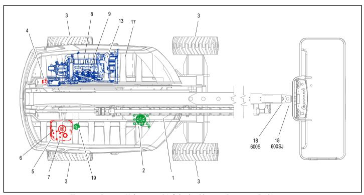
Figure 7-6. Operator Maintenance & Lubrication Diagram - Deutz 2011 Engine
