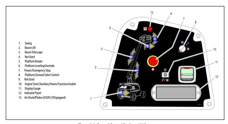
Figure 3-1. Ground Control Station - 600S
