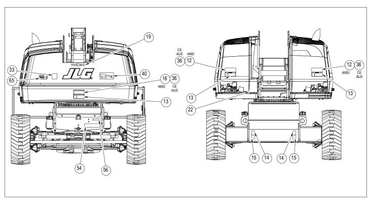
Figure 4-10. Decal Installation - Sheet 3 of 6
