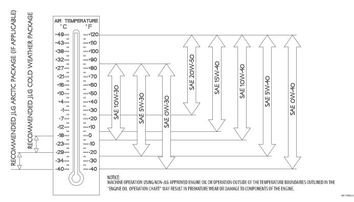
Figure 7-2. Engine Operating Temperature Specifications - Deutz 2.9L
