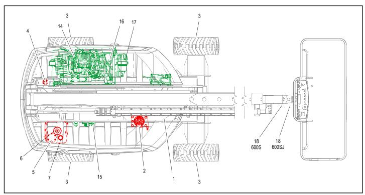
Figure 7-8. Operator Maintenance & Lubrication Diagram - Ford Engine
