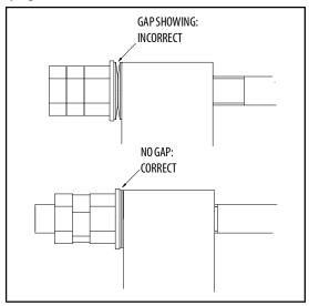
Figure 6-4. Bolt-On External Fall Arrest Cable Tension
