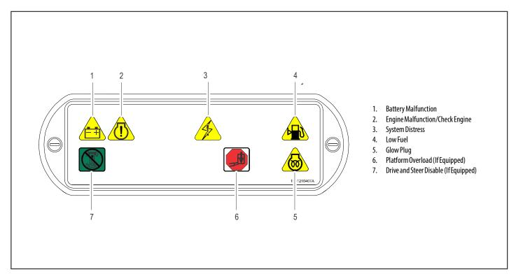
**Figure 3-5. Ground Control Indicator Panel**
