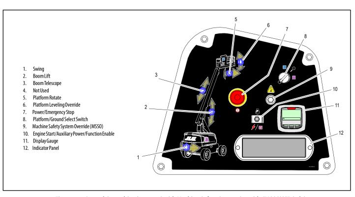
Figure 3-2. Ground Control Station - 600S with Machine Safety System Override (MSSO)(CE Only)
