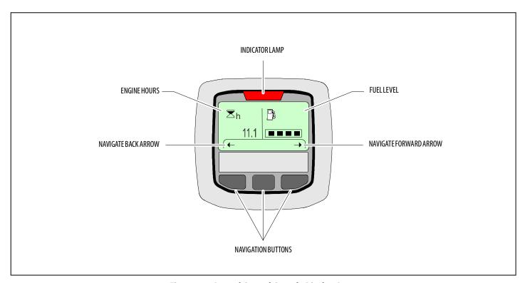
Figure 3-9. Ground Control Console Display Gauge
