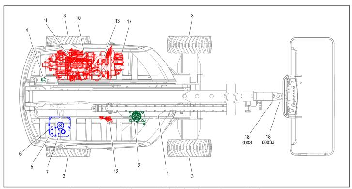
Figure 7-7. Operator Maintenance & Lubrication Diagram - Deutz 2.9L Engine
