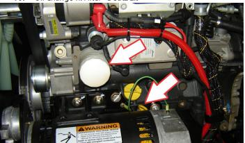
Lube Point(s) - Fill Cap/Spin-on Element Capacity - 9.5 Quarts (9.0 L) Crankcase
