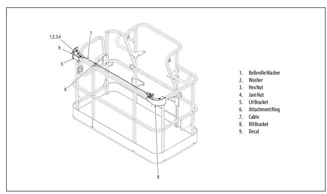
Figure 6-5. Bolt-On External Fall Arrest System
