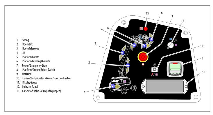
Figure 3-3. Ground Control Station - 660SJ
