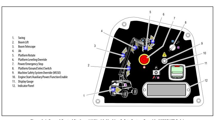
Figure 3-4. Ground Control Station - 660SJ with Machine Safety System Override (MSSO)(CE Only)
