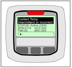
Figure 3-8. Engine Diagnostic Screen
